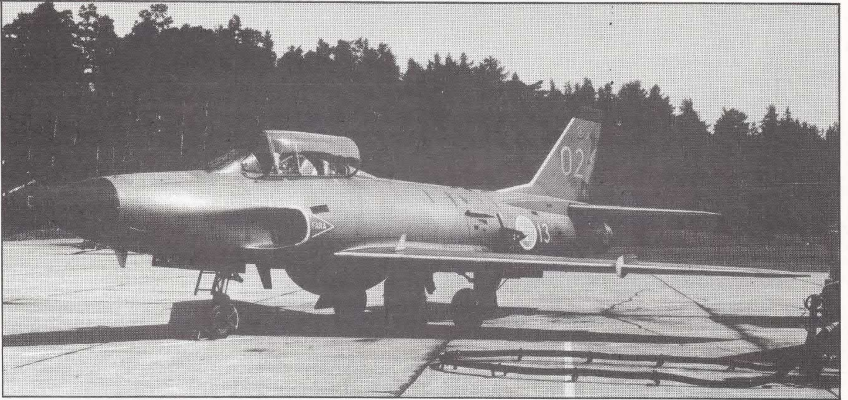
SAAB J-32D 13-02, the J-32D is the target towing version of the Lansen. The code '13' refers to the squadro
